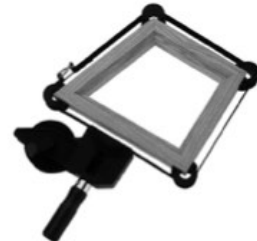
BAND CLAMP Art. 15388 Tape length 700 cm. complete with 4 corner inserts. Winding me- chanism with crank and automatic locking during tightening.
