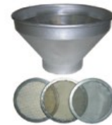
ALUMINIUM SIEVES For powders and liquids. Supplied with 3 brass nets, meshes other interchangeable. 1 x 1 - 0.5 x 0.5 - 0.1 x 0.1 mm Art. 15041 Ø 15 x 7 cm. Art. 15044 Ø 27 x 13 cm. Art. 15042 net sapre for Art.15041 Art. 15045 net sapre for Art.15044
